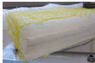
Multilayer Vliesmuster aus OilSepTIN (PP-Nadelvlies) und PP-Meltblown-Vlies
